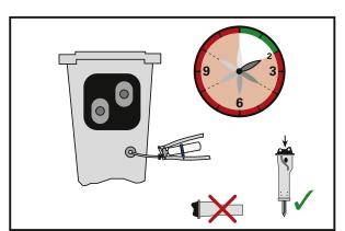
Reposition the demolition tool at regular intervals during operation to avoid overheating of the material.
