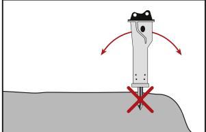
Try to avoid bending stresses on demolition tools at all times to avoid overstressing of the material.
