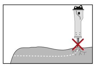
Demolition tools should always be positioned at right angles to the working surface to avoid long-term secondary damage.
