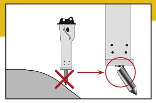
Rock the breaker gently during operation to allow the dust to escape from beneath the tip of the demolition tool, and never attempt to use the hydraulic breaker as a crowbar.
